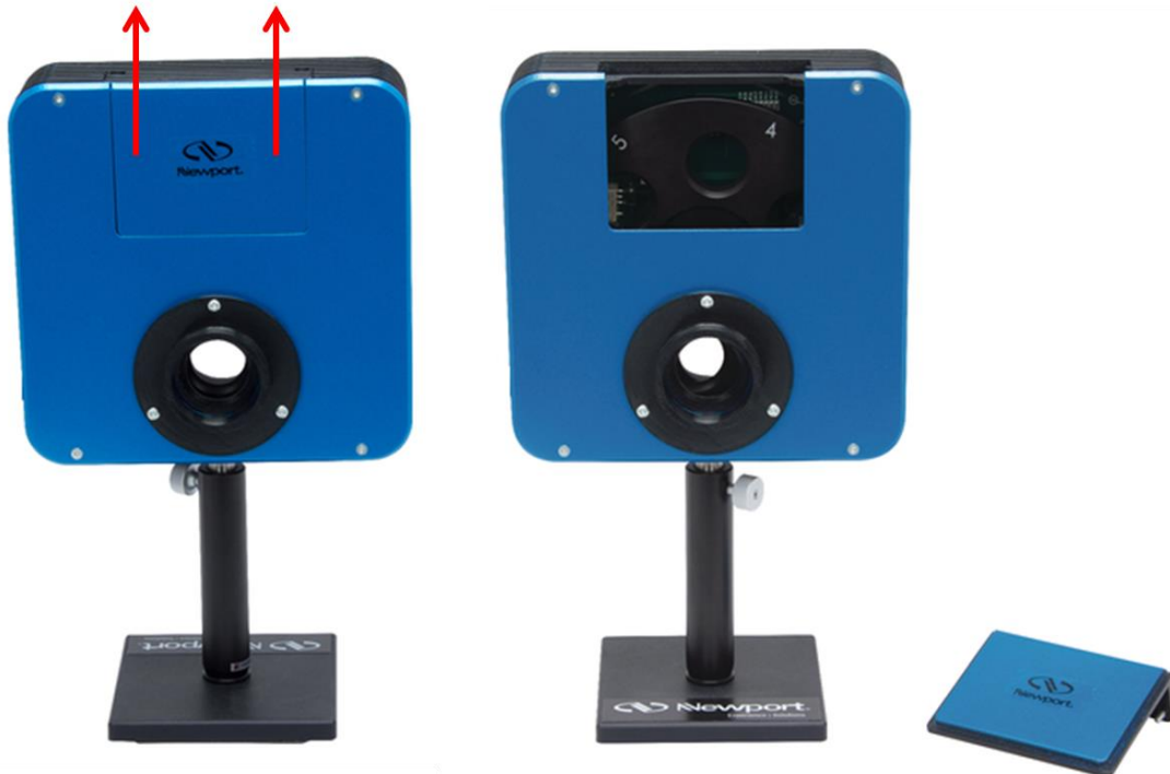
Figure 3: Removing the access plate to add/remove filters
