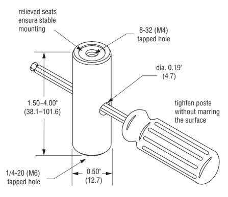
our posts have cross-drilled holes for better leverage (ball driver not included)
