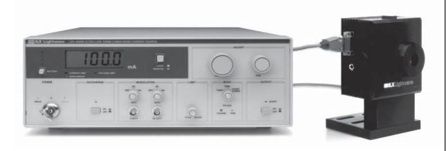
The LDX-3620B is compatible with a large selection of laser diode mounts. Shown is the LDX-3620B with an LDM-4412 TO-Can laser diode mount.
