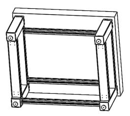
1. Adjust the leveling feet so that the caster can fit underneath the frame
