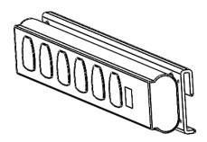
2. Attach the mounting bracket to the desired location on the Integrity VCS overhead shelf. Tighten screws under the bracket to secure the bracket to the shelf.
