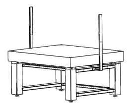
Have a colleague assist with lifting the shelf assembly into position and attachment hardware to fasten shelf to the uprights. Make sure all connections are secure by tightening down the bolts.
