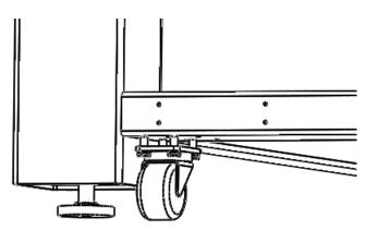
2. Bolt the casters underneath the frame on the sides. Check to make sure all the connections are secure. Readjust leveling feet height if needed.
