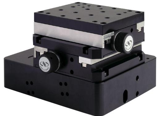
Ultra low-profile precision XYZ system consisting of two VP-25XA linear stages and one VP-5ZA vertical translation stage. Compared to traditional stacks of stages, this solution offers a lower-profile alternative with easy access to the load from any side.
