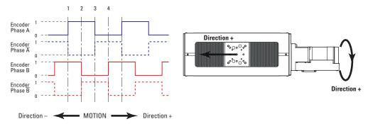
The incremental sensor consists of an optical scale and an encoder head. When the carriage moves, the encoder head generates square signals in quadrature and sends to pins #19, #20, #23 and #24 of the SUB-D25 connector.
