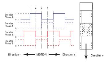
The incremental sensor consists of an optical scale and an encoder head. When the carriage moves, the encoder head generates square signals in quadrature and sends to pins #19, #20, #23 and #24 of the SUB-D25 connector.
