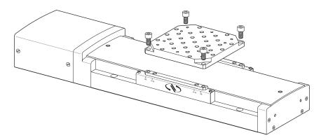
To do that, just unscrew the 4 CHc M6 x .47 (12) on SQR 3.94 (100) screws at the 4 corners of the plate with the wrench supplied with the stage. Both ILS and M-ILS stages will then have the same following interfaces:
