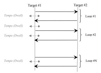
In the "Target Motion / PA" area, two target positions can be defined. The "Go to" button executes the absolute move to go to the specified target position.
