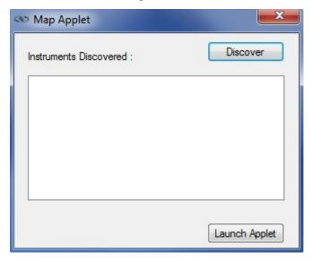
Next, click on "**Discover**" and the number of stages discovered will appear. This window allows the user to select a COM port where the desired stage is connected.
