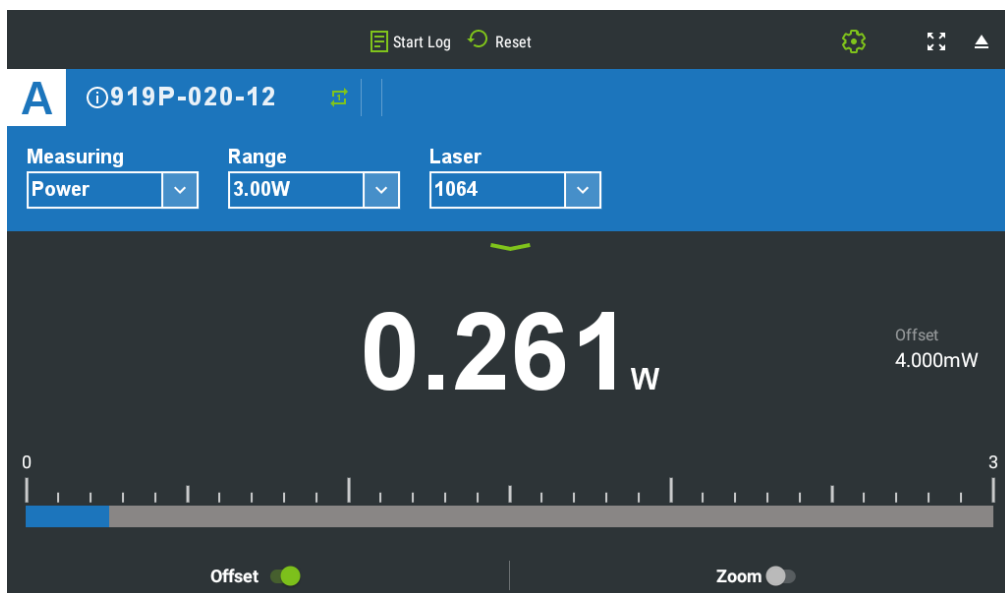
Figure 4-21 Photodiode Bargraph showing stored offset
