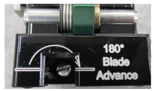
Advance blade to next position by turning screw head
