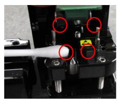
Keep clamping ridges, rubber clamps and blade **CLEAN** or the fiber strength will be reduced. Use alcohol-soaked, lint-
