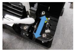
Dust may damage the blade. Wipe alcohol-soaked, lintfree swab along blade.
