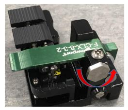
To open cleaver, rotate hexagonal latch as shown
