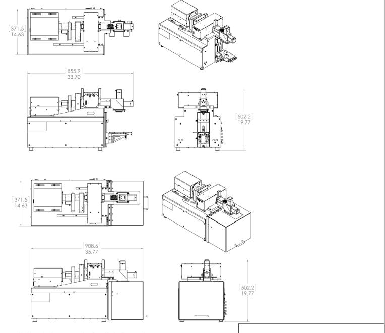
Note that the actual monochromator used in this product is not accurately reflected in the diagrams above, but the overall system dimensions remain unchanged.
