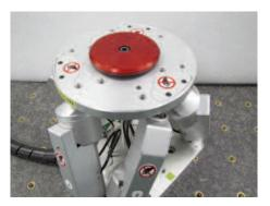
To avoid damages, the HXP50-MECA Hexapod is delivered with a locking system that includes a center rod and a clamping wheel.
