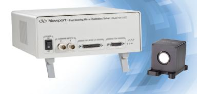
The Fast Steering Mirror Series provides two-axis, high-bandwidth rotation with sub-microradian mechanical resolution using voice-coil technology. Utilizing a unique flexure suspension design to confine the motion of the mirror results in ultra-smooth motion about a gimbal point, very high accuracy, and practically no wear. Newport offers a wide range of 1" field replaceable mirrors.
