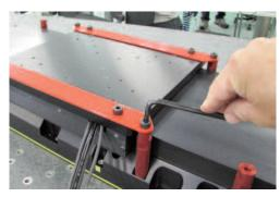
③ Unscrew with the supplied Allen key, 4 CHc M6 screws from the 2 locking brackets on the carriage.
