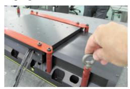
(2) Unscrew with the supplied Allen key,4 CHc M8 screws from the 2 locking brackets on rods.
