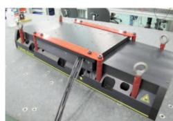
① Unscrew the lifting rings fixed on the rods.
