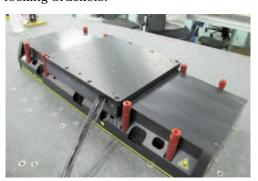
(5) Unscrew and remove 8 mounting rods of the lifting rings and the locking plate.
