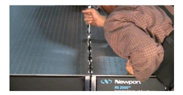
After all the bolts are uniformly engaged and table sections are in full contact use the recommended staggered tightening sequence to apply a final torque of 60 ft-lbs (80Nm) to all bolts. This sequence helps ensure uniform torque loading and proper mating of the plate. It is important that this sequence be followed carefully.
