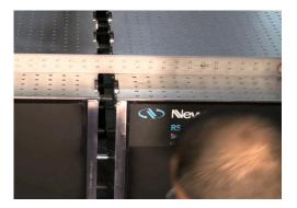
Carefully move the two sections together close enough so they can be leveled and aligned to allow the guide pins and bolts to mate to their respective holes. Be very careful of any potential pinch points as the sections come together. It is recommended to use a 48" or longer level across the joint, to assure both table sections are at equal heights and level.
