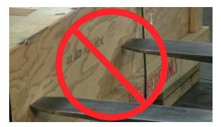
Under no circumstances should you attempt to use a forklift or other blunt tool to push or lift the crate along its sidewall or top as this may result in damage to the table.
