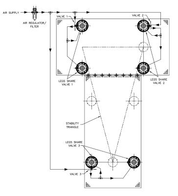
In this final example a "T-Shaped" doubler system (shown on page 7) is shown being supported by six S-2000 isolators. As in the previous example each leveling valve controls two isolator legs and in this configuration the pairs of legs at the outermost sections of the table are controlled by Valves 1,2 and 3. This creates the largest stability triangle possible for this system shape.
