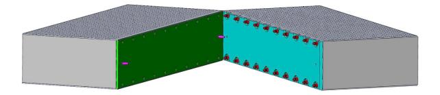
Refer to the recommended bolt torque sequence in the installation guide and if needed note the recommended sequence on the table surfaces using a pencil prior to joining the sections. This will help guide the order in which the bolts should be torqued after initial hand-tightening to ensure uniform mating and reduce the risk of improper alignment.
