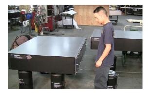
final assembly. Also, be certain that the matched sets are being assembled correctly for multi-section table systems. Contact Newport if there are any components that may look damaged for repair instructions.
