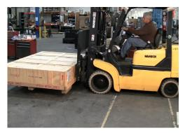
Use proper lifting and maneuvering techniques to move the table to its unpacking location. This includes lifting the crate from the bottom and only pushing against designated areas when necessary.
