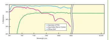
Our integrating spheres are available with PTFE (spectralon), barium sulfate (spectraflect), and diffused gold sphere materials.
