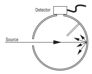
819C integrating sphere configuration is ideal for a collimated beam source such as a collimated laser beam.
