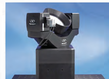
High speed 2-axis motion simulator using RGV series for continuous 360° rotation, speeds up to 720 °/s, high acceleration, 0.001° MIM for MEMS-based inertial sensors testing. ▶
