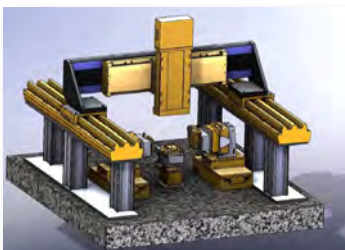
◀ 24 axis system for alignment of a variety of telcom devices, built from standard stages. The system includes pick and place capability of optical components.
