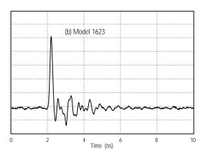
A 0.15-ps pulse at 1.06 µm was used to test the photodetectors, and the output was measured using a 12-GHz oscilloscope.
