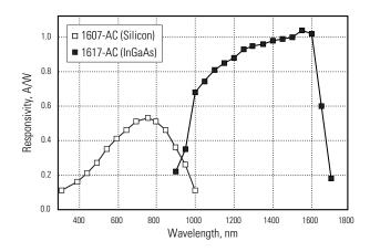
The amplifier has a maximum input current of 2 mA; to avoid damage to the amplifier, never exceed this input current. The Model 1607-AC has a peak responsivity of 0.5 A/W, which means that 2 mA of photo-
