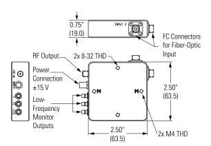
Transmission lines connect the photodiode to the amplifier and the amplifier to the output. The transmission lines help to preserve speed and reduce parasitic inductance and capacitance that can cause ringing. DC power is delivered to the balanced photoreceiver through a microconnector on the side of the unit, and the entire package is shielded to eliminate noise pickup.
