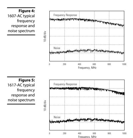
From 40 kHz to 800 MHz the integrated input noise current is approximately  $1.5 \,\mu A_{rms}$ . Multiplying this by the 700-V/A transimpedance gain gives an output voltage noise of  $1.1 \, mV_{rms}$ .
