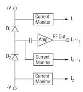
Figure 1: Functional block diagram of the Model 16X7-AC
