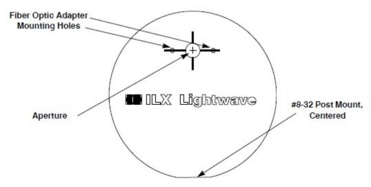
Figure 2.4 - OMH-6742B Optical Measurement Head
