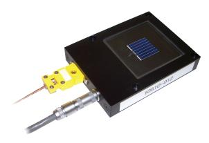
Each reference cell is provided with a certificate which is accredited by A2LA to the ISO 17025 standard and is traceable both to the National Renewable Energy Laboratory (NREL) and to the International System of Units (SI). It reads solar simulator irradiance in Sun units, where one sun is equal to 1000 W/m² at 25°C and Air Mass 1.5 Global reference.
