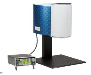
is rigorously tested for all aspects of the standards to ensure compliance. The innovative design independently drives multiple LEDs at nineteen individual wavelength bands, from 400 nm to 1100 nm, to ensure a spectral match. The independent control of each LED allows for custom tuning of the output to the specific requirements of a test.
