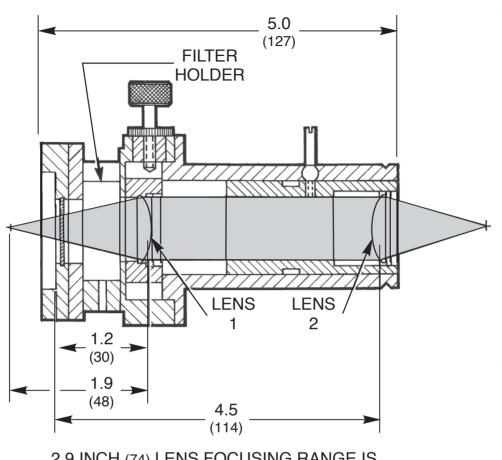
2.9 INCH (74) LENS FOCUSING RANGE IS AVAILABLE WITH VARIOUS LENS POSITIONS
